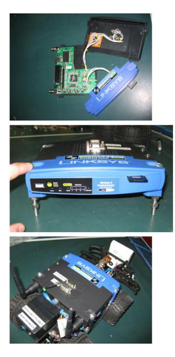
I've modified my WRT54GL to have 2 serial ports and a 1GB SD Card (acts like a 1GB hard drive). The SD card is not used in this project, but one of the serial ports is. One is a console port, the other is TTS/1 which we will be using. For this project I'm using Open-WRT White Russian v0.9. There are more recent versions, but we don't need the latest-and-greatest software features for this project. The software compilation guide (details later) uses this distribution, so that is why I chose it.
