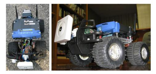
All of the electronics were prototyped on a breadboard before being soldered and installed in the car. The batteries were secured using hot-glue and zip-ties. The router was a bit too wide
