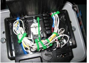
All of the power electronics are on a prototype board and are stored under a project box.
