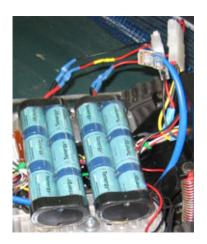
This project sucks some major battery power. I bought some high-end RC car batteries for about \$50+shipping on eBay. They're 3800mAh and came with a 1.8A smart charger. They can be found with this <u>eBay search</u>. Each battery takes about 1.5hrs to charge (from being completely dead). They're 7.2V, however when they're just-charged they're ~8.3V and when they're dead (no longer able to move the car) they measure ~7.1V.
