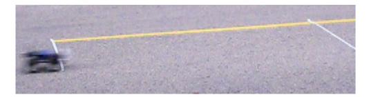
The car could travel 3m in 0.7 seconds (21 out of 30 frames in 1 second). **Top Speed:** 4.3m/s = 15.5km/h = 9.6miles/h
