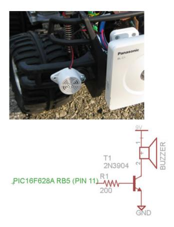
I wanted to add the fun feature of being able to honk at people. It was a pretty simple addition. I bought a \$3 buzzer for KW Surplus and hooked it up to the microcontroller using a transistor for greater voltage and current.
